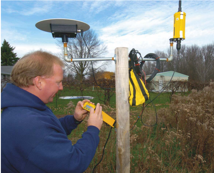
Chrisman checks one of two base stations that his company maintains. The base station is a fixed, known reference point that communicates via radio with the GPS grade-control system to improve the accuracy of blade control.
